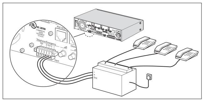
figure 4.5: Connecting emergency telephone lines
